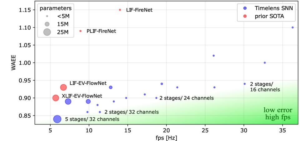
**Model reduction results:** Our model (blue) compared with prior state-of-the-art (SOTA) [4] (red) in our CPU setup. **Optical Flow quality** (WAAE) is plotted vs. **frames per second** (fps) while circle size indicates model size.
