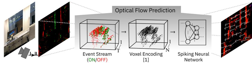
We propose an architecture that can operate both in a spiking and a non-spiking mode. **Model simplification** based on activity and latency analysis is performed to demonstrate high speed optical flow prediction for **real-time** deployments.
