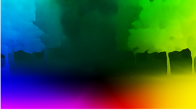
Figure 5. Example flow prediction on the car_urban-parking sequence using E-RAFT (color represents direction). The high-resolution events allow rich details to appear in the flow results. Color denotes the direction of the flow at each pixel. Best viewed in color.
