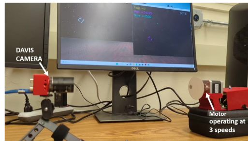
Figure 2. Experimental setup to demonstrate speed detection using DOTIE. The event camera is used to capture the events generated by a disk attached to a motor rotating at three different speeds.
