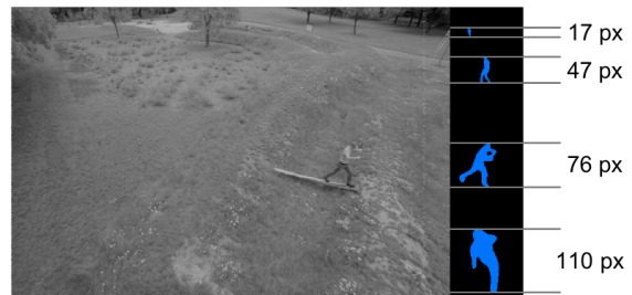
(d) FoV from DVS1 as greyscale image for clarification with typical object heights for an adult person depending on the distance to the sensor
